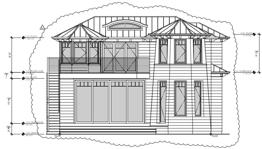
2 SOUTH ELEVATION SCALE: 1/4" = 1'-0"
