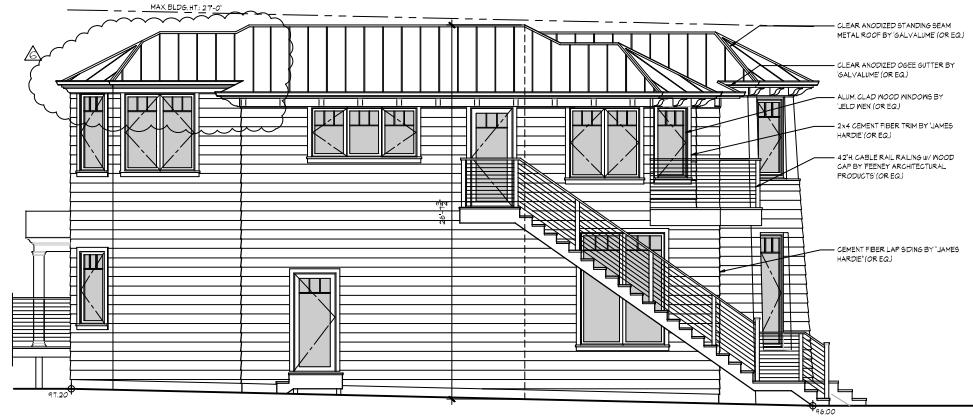
2 EAST ELEVATION SCALE: 1/4" = 1'-0"
