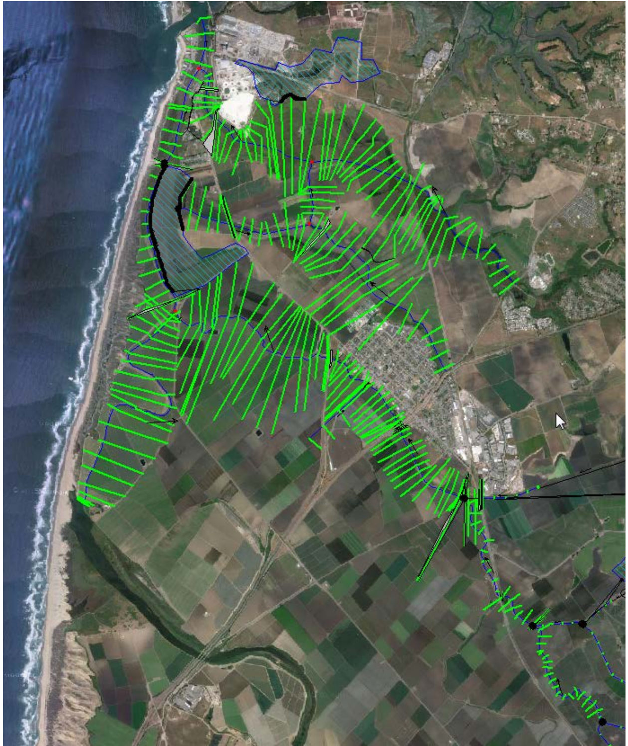
Figure 8. Reclamation Ditch hydraulic model layout
