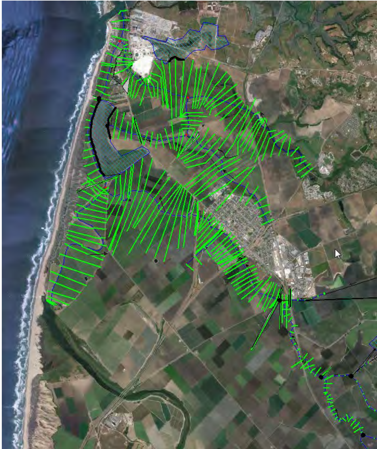
Figure 8. Reclamation Ditch hydraulic model layout
