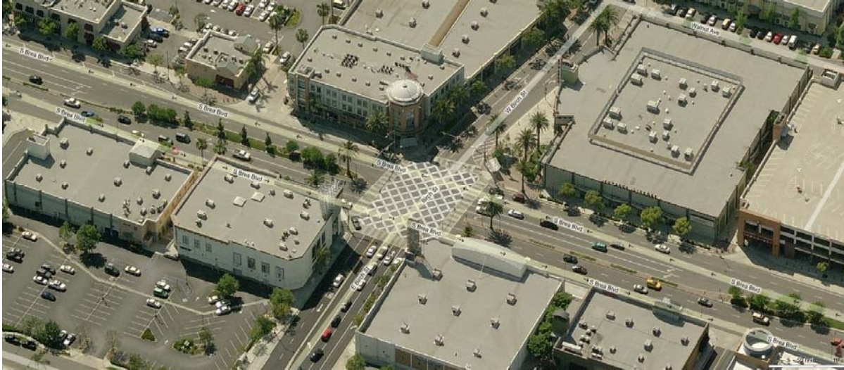
Birds-eye view of Brea Boulevard (running left to right) and perpendicular Birch Street. Notice the buildings constructed up to the sidewalk, the all-direction “scramble” pedestrian crosswalk, and that pedestrian-oriented is concentrated along both sides of Birch Street, rather than busy Brea Boulevard. Source: Microsoft Bing Maps, 2011.
