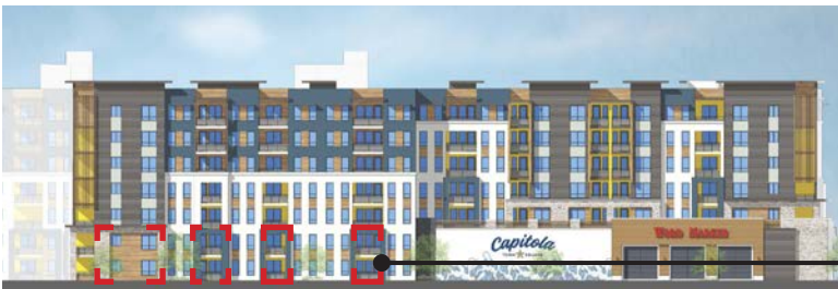
Residential portion of project lacking adequate pedestrian-scaled elements. Introduce additional, appropriately scaled two- and three-story elements to break down monumental mass of buildings.
