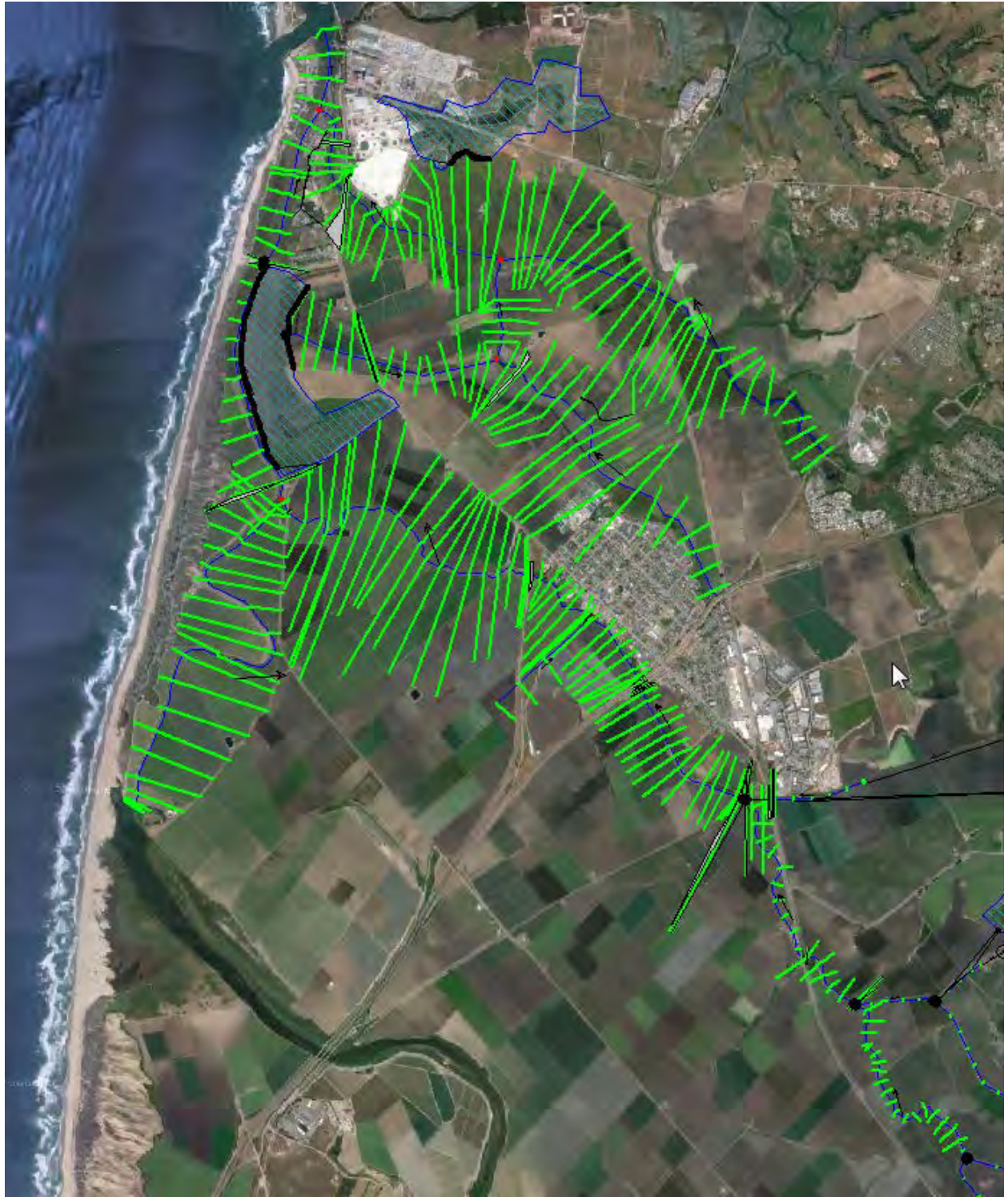
Figure 8. Reclamation Ditch hydraulic model layout
