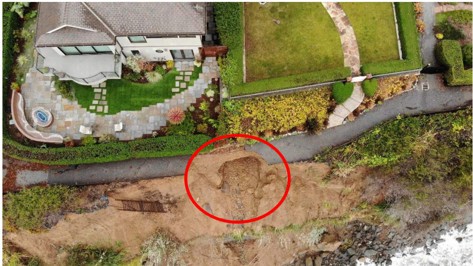
Runoff draining into area of slope failure
