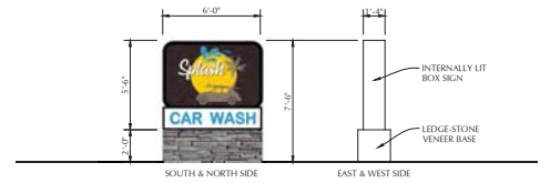
2 PROPOSED MONUMENT SIGN SCALE: 1/4" = 1'-0" SIGNAGE AREA CALCULATION = 1 S.F. PER 1 L.F. OF FRONTAGE. 50 S.F. MAX EXISTING FRONTAGE = 114 L.F. > 50 S.F. = MAXIMUM ALLOWED PROPOSED SIGN AREA PER SIDE = 33 S.F.
