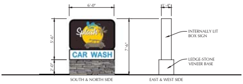
2 PROPOSED MONUMENT SIGN SCALE: 1/4" = 1'-0" SIGNAGE AREA CALCULATION = 1 S.F. PER 1 L.F. OF FRONTAGE, 50 S.F. MAX EXISTING FRONTAGE = 114 L.F. = 50 S.F. = MAXIMUM ALLOWED PROPOSED SIGN AREA PER SIDE = 33 S.F.
