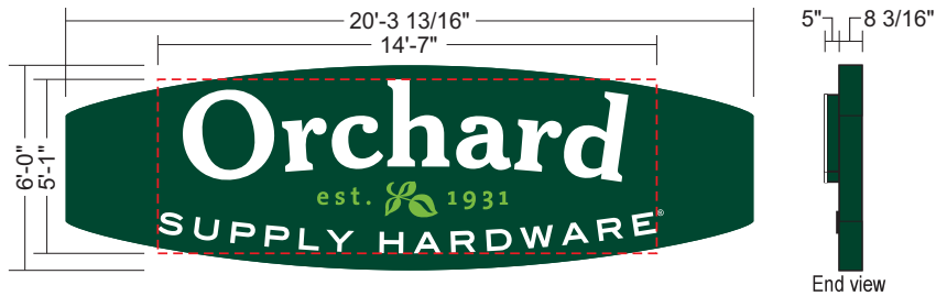
A TRADEMARK SKATEBOARD SPECIFICATIONS Scale: 1/4" = 1'-0" Manufacture and install one (1) 6'-0" OAH trademark skateboard sign
