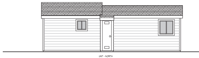
4 EXISTING NORTH ELEVATION SCALE: 1/4" = 1'-0"
