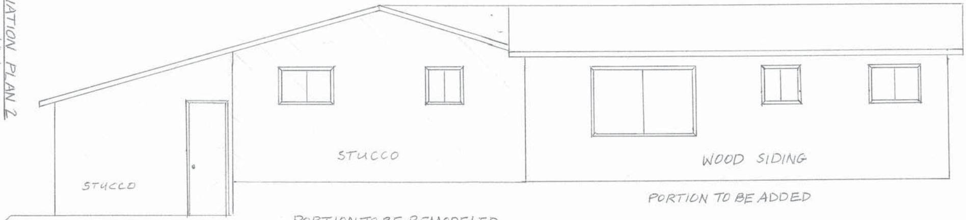
STUCCO WOOD SIDING PORTION TO REMAIN AS BUILT PORTION TO BE REMODELED PORTION TO BE ADDED SOUTH ELEVATION
