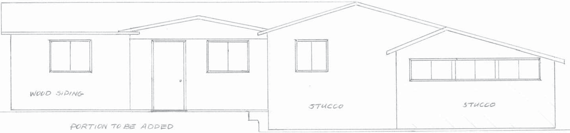
WOOD SIDING STUCCO STUCCO PORTION TO BE ADDED PORTION TO REMODEL PORTION TO REMAIN AS BUILT NORTH ELEVATION
