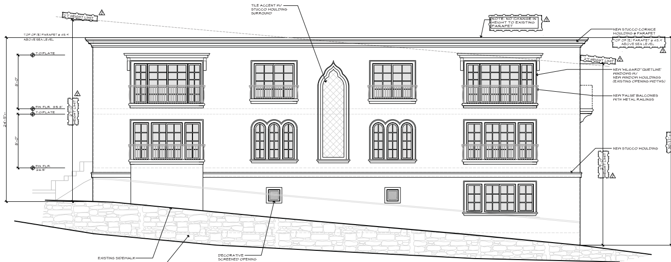
1 EXISTING WEST ELEVATION 1/4" = 1'-0" AVERAGE EXISTING BUILDING HEIGHT = 25.5'
