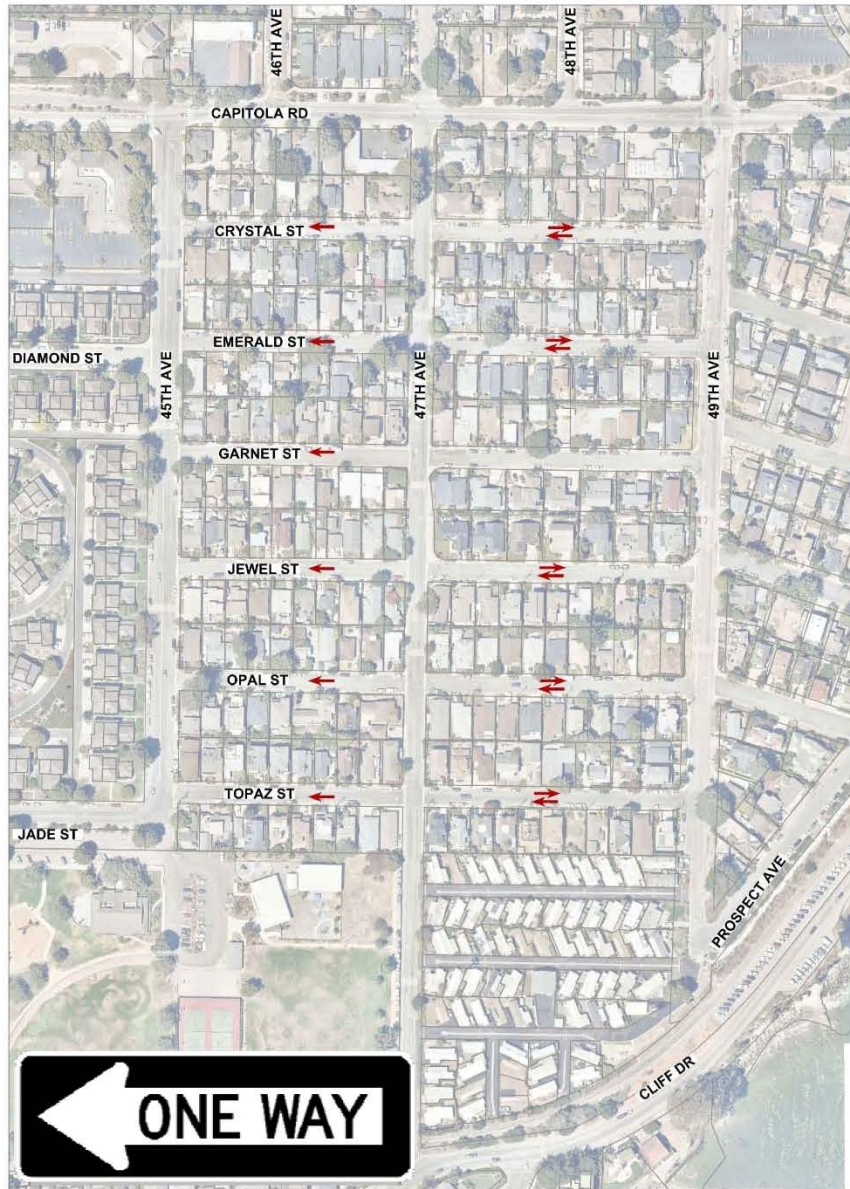
TRAFFIC CALMING ALTERNATIVE: PARTIAL ONE-WAY WEST SIDE
