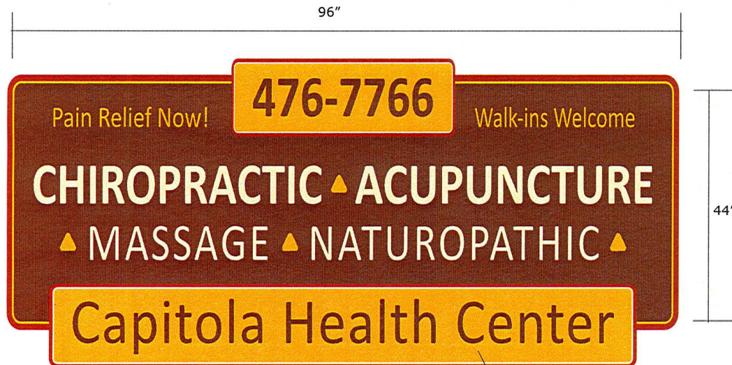
1/8" COMPOSITE ALUMINUM/PVC PANEL WITH DIGITALLY PRINTED GRAPHICS
