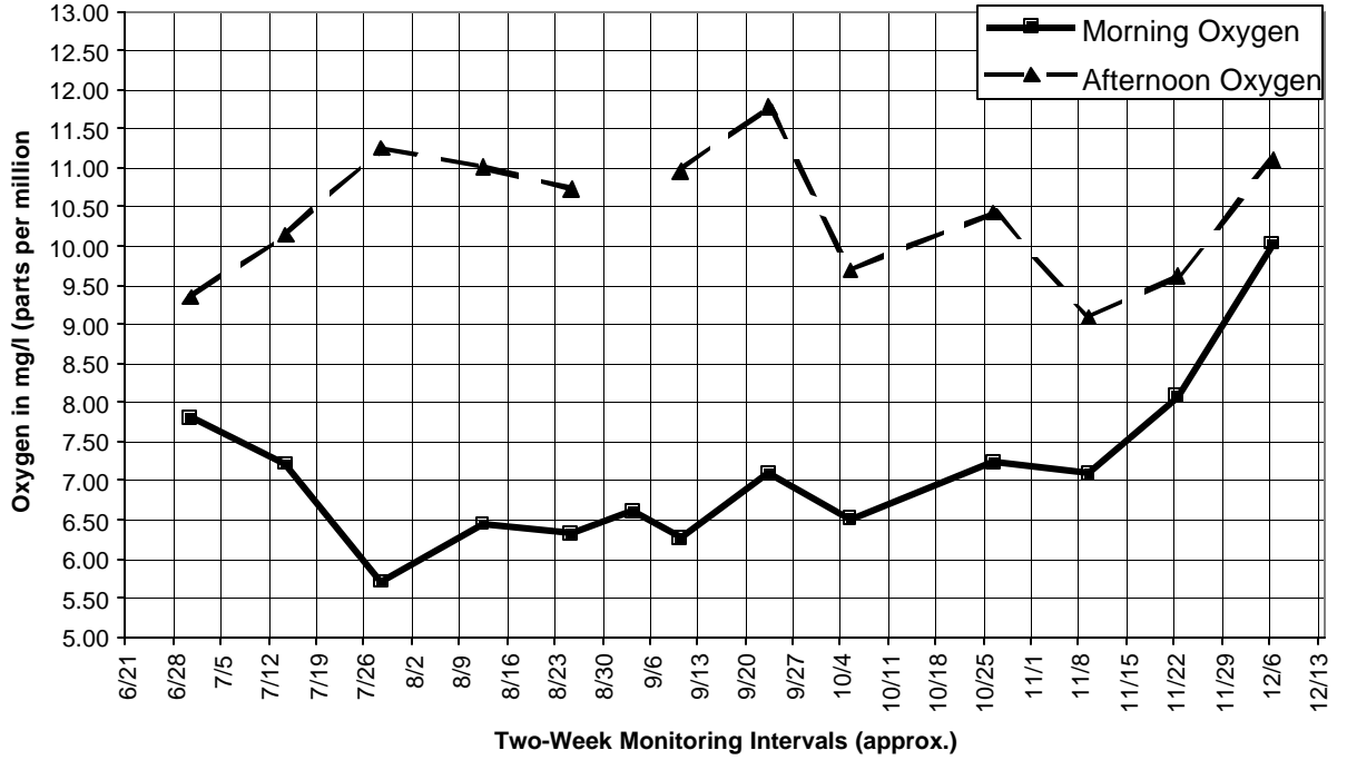
Figure 6j. Soquel Lagoon Oxygen Concentrations in the Morning and Afternoon Within 0.25 Meters of the Bottom at Station 4, the Mouth of Noble Gulch, 30 June - 6 December 2006.
