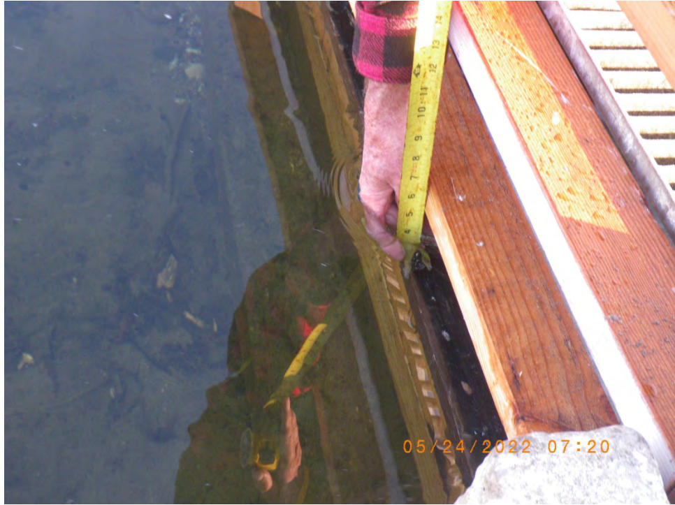
Lagoon spilling over base of the wooden frame, with smolt passage previous night. 24 May 2022
