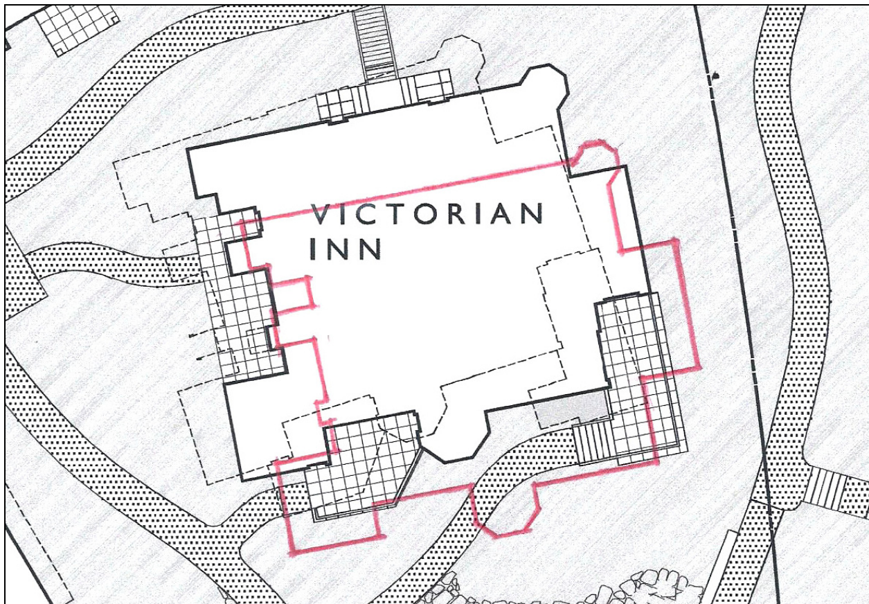
Figure 4. Marked-up version of project site plan (Appendix C) showing current location of Main House (in dashed line), temporary location (in red line), and final location (in solid black line). Charles Eadie of Hamilton Swift and Associates submitted this graphic to ARG on August 16, 2013.
